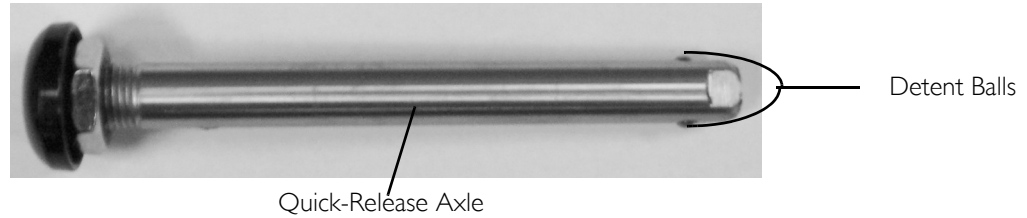
FIGURE 7.2 Adjusting Quick-Release Axle
